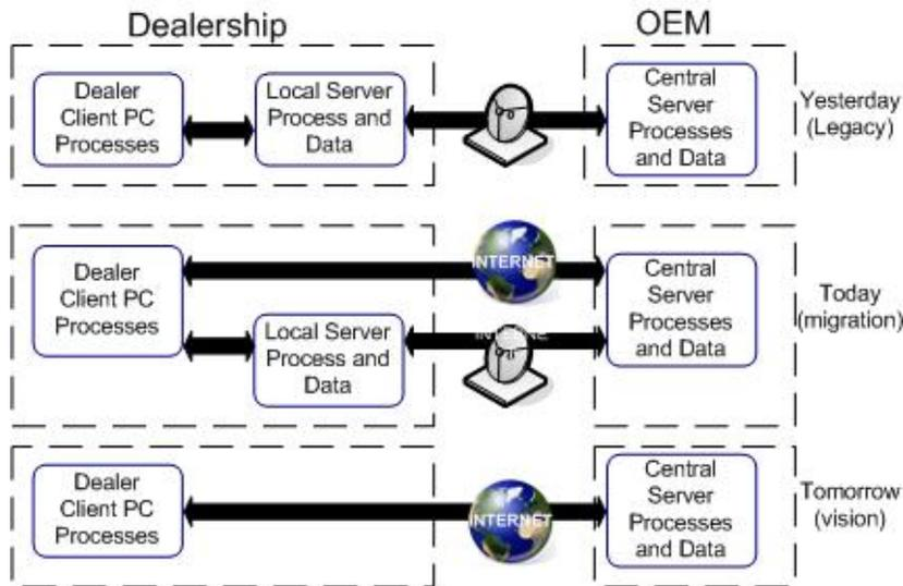
An external path to the data on the central server is required. Due to the volume of traffic required for dealership applications, the existing link to OEMs using the current satellite technology may not be adequate. Even small dealerships might find the delay of the medium unacceptable. That leads to the need to communicate over a faster and larger medium. The most likely choices include telephone services like a Digital Subscriber Line (DSL) and a T1.
