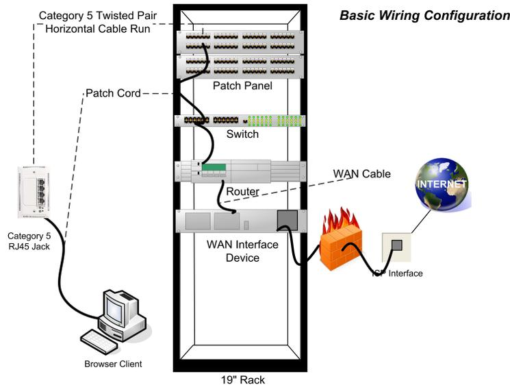
A sample wiring configuration is demonstrated above (see Figure 2.1, “Simplified Dealership Wiring”). This diagram represents the base configuration that allows a Personal Computer (PC) in the dealership to access the Internet. Dealer Management System (DMS) equipment, any satellite or OEM-specified equipment, and other dealership installed equipment comprising the remainder of the entire dealership network are not shown on this diagram.
