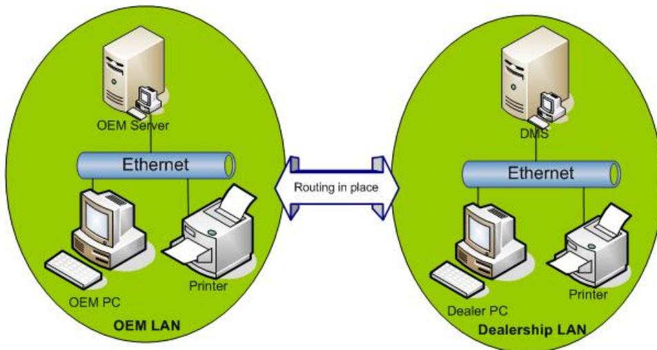
Routers with logical sub-interfaces contained on a single physical Ethernet interface can route traffic between sub-networks that exist in a switched environment. This allows traffic to pass or be filtered depending on the situation. Routers with multiple physical Ethernet interfaces can be used for non-switched and switched environments. Use routers with these capabilities to communicate between different sub-networks in a local environment.
